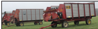
Left to Right: NH 18' Tandem S/U 3 Beater Roof Meyer 3516 18' 3 Beater, H&S 16' 2 Beater
